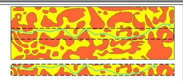
Probing current (blue arrow) in an unconfined structure (top) will follow the path of least resistance. Confining the conduction path (bottom) allows probing electrons to gather previously hidden data.
