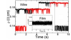
Discrete jumps in resistivity indicate that single electronic phase domains are actively fluctuating between electronic phases. Red and black plots were taken 5 hours apart and indicate the robust nature of the system. This behavior is never seen in the film geometry, as single domain fluctuations are drown out by the larger system.
