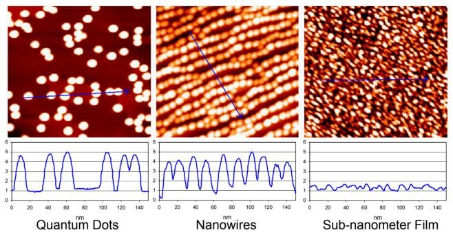
Above: Atomic force microscope images of quantum dots, nanowires, and and an ultrathin film formed from 1.7 atomic layers of iron on a cleaved NaCl (100) surface. Each image is 200 nm x 200 nm. The blue linescan under the image to the left shows the height and surprising uniformity of the dots, which could be important for technological applications.
