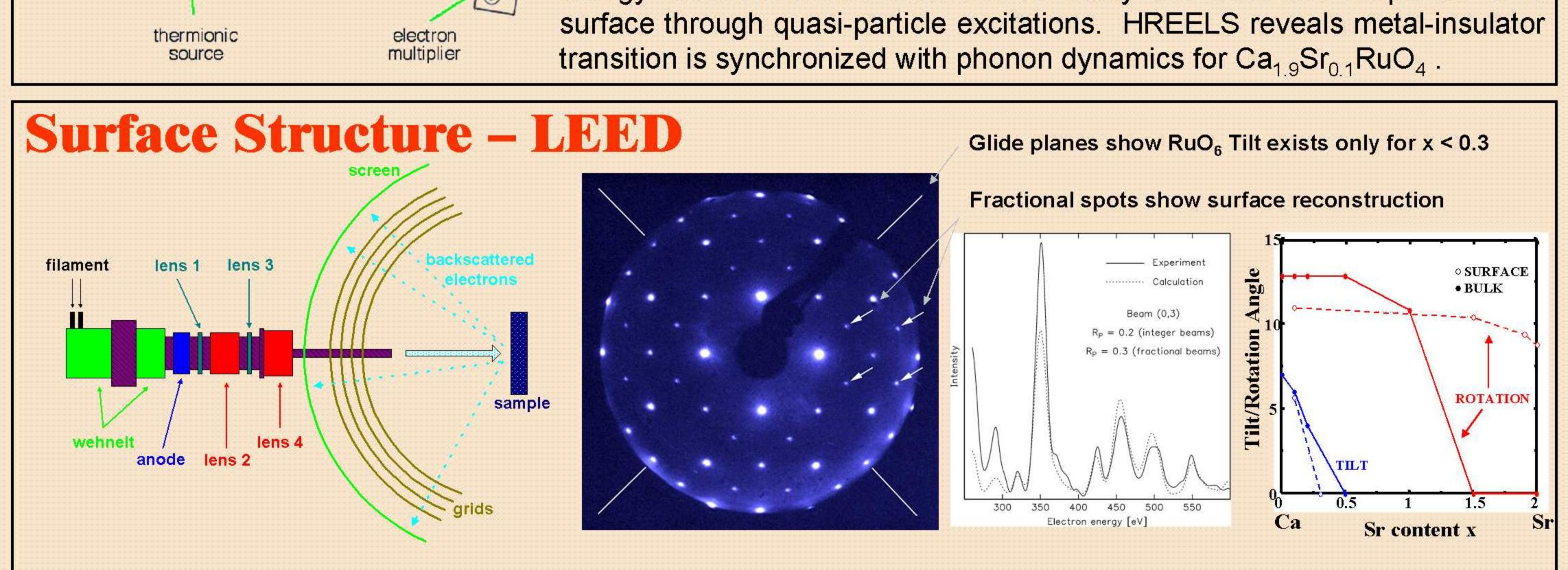
Low Energy Electron Diffraction (LEED) reveals the surface structure of the crystals. By tracking diffraction spots as a function of incident electron beam energy (LEED-IV), surface reconstruction can be calculated to determine the rotation and tilt of the RuO<sub>6</sub> octahedra.
