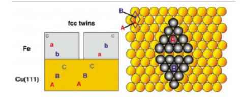
Schematics showing the phenomenon of twinning. The spacing between iron atoms on the Cu(111) surface is such that iron atoms in a particular island will either occupy 'A' sites only or 'B' sites only, depending on which of these two sites was settled upon by the atom that seeded the island. The image shows the fault line that forms when an A-type island tries to merge with a B-type island.
