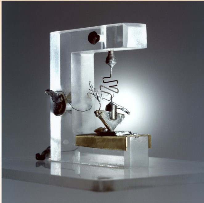
First Transistor, 1947 (Bell Labs)
