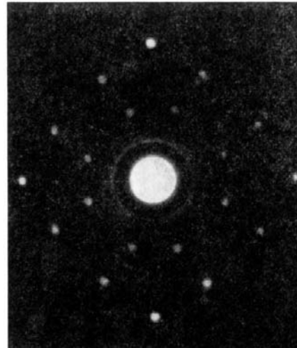
FIG. 1. Laue photograph showing neutron diffraction by NaCl.
