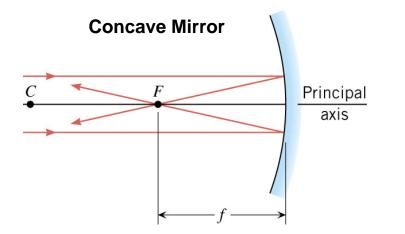
For the concave mirror, the parallel rays get reflected thru the focal point.  $\rightarrow$  The image is <u>Real</u> (rays come from the image)
