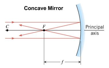
For the concave mirror, the parallel rays get reflected thru the focal point.
