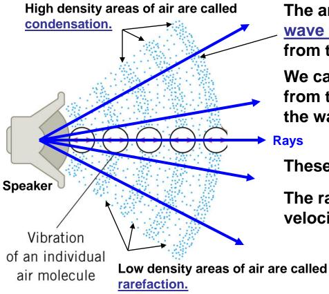
The areas of condensation are also called wave fronts, and they propagate out away from the source.
