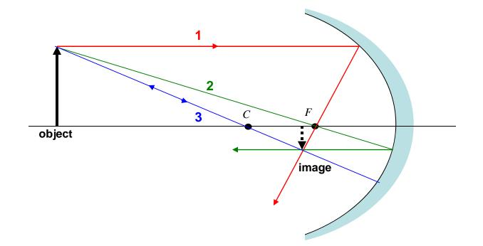
So now I can see where the image is located – at the intersection of the reflected rays!
