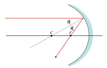
When a paraxial ray comes in, it reflects off the surface and pass thru *F*.
