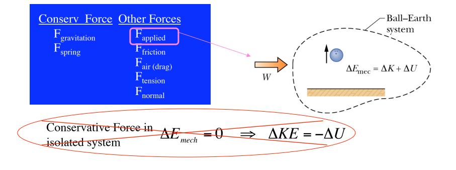
If External force: $W_{ext,net} = \Delta E_{mech} = \Delta KE + \Delta U$ (NO FRICTION)Positive if energy is transferred to systemNegative if energy is transferred from system
