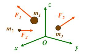
$M\vec{a}_{com} = m_1\vec{a}_1 + m_2\vec{a}_2 + m_3\vec{a}_3 + \dots + m_n\vec{a}_n.$ We apply Newton's second law for the *i*th particle:  $m_i\vec{a}_i = \vec{F}_i.$  Here  $\vec{F}_i$  is the net force on the *i*th particle,  $M\vec{a}_{com} = \vec{F}_1 + \vec{F}_2 + \vec{F}_3 + \dots + \vec{F}_n.$
