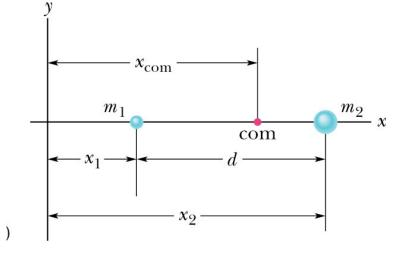
$$\begin{aligned} x_{com} &= \frac{m_1 x_1 + m_2 x_2}{m_1 + m_2} \\ y_{com} &= \frac{m_1 y_1 + m_2 y_2}{m_1 + m_2} \\ &= \frac{m_1 (0) + m_2 (0)}{m_1 + m_2} = 0 \\ Note: Use symmetry! \end{aligned}$$
