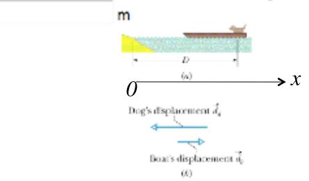
Step I: choose a system  $\Rightarrow boat(m_b) + dog(m_d)$ Step II: Find net force  $F_{net}^x = 0 \Rightarrow$  COM remains unchanged
