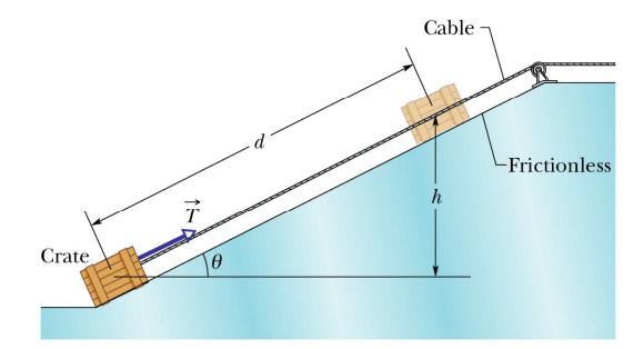
An initially stationary crate of cheese (mass m) is pulled via a cable a distance d up a frictionless ramp of angle  $\theta$  where it stops.
