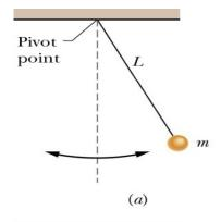
2) Simple Pendulum: gravity is "restoring force"
