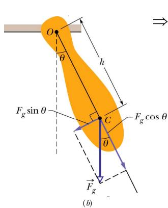
**15-49:** A stick of length L oscillates as a physical pendulum. (a) What value of distance x between the stick's COM ant is pivot point O gives the least period? (b) What is the least period?
