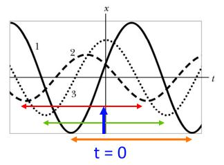
x(t) curves for the experiments involving a particular spring-box systems oscillating in SHM (equal k's).
