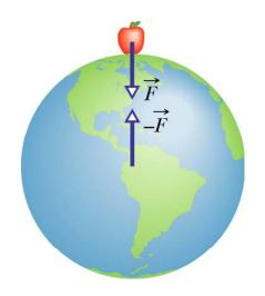
A uniform shell of matter exerts no net gravitational force on a particle located inside it.
