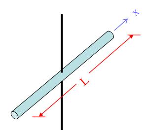
**Example:** moment of inertia of thin rod with perpendicular rotation through center
