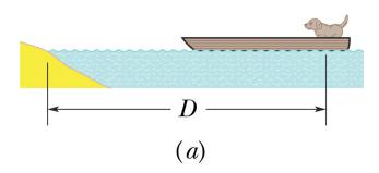
Step I: choose a system  $\Rightarrow boat(m_b) + dog(m_d)$ Step II: Find net force  $F_{net}^x = 0 \Rightarrow$  COM remains unchanged
