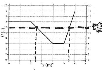
(B) (5pts) What is the allowed range of the motion along x given the mechanical energy found above (hint: you can read this off of the graph)?
