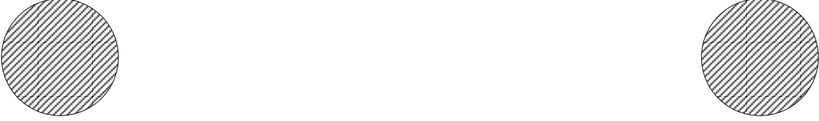
Figure 4: Two isolated orbitals. If they are far apart, each has a Hamiltonian H_0 = \epsilon n , where n is the orbital occupancy.
