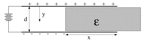
**Part b.** The battery is disconnected from the capacitor *before* the dielectric is inserted, leaving the capacitor charged. Then the dielectric is inserted. Now what are the answers to five questions above?
