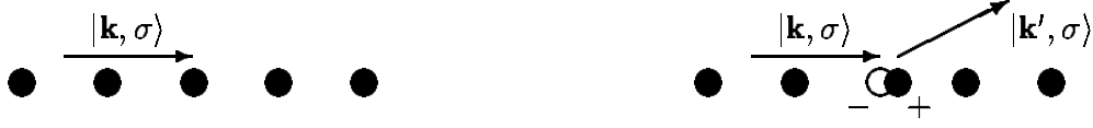
Figure 3.8: (a) Being in an eigenstate a Bloch electron moves through a perfect lattice without being scattered. (b) A displaced ion results in an electric dipole relative to the perfect background, and this can scatter Bloch electrons from |\mathbf{k}, \sigma\rangle to |\mathbf{k}', \sigma\rangle .
