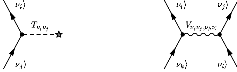
Figure 1.5: A graphical representation of the one- and two-particle operators in second quantization. The incoming and outgoing arrows represent initial and final states, respectively. The dashed and wiggled lines represent the transition amplitudes for the one- and two-particle processes contained in the operators.
