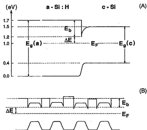
FIG. 1. Energy-band diagrams for (A) *a*-Si:H/*c*-Si heterojunction [the band gap of *c*-Si is  $E_g(c) = 1.1$  eV, the band gap of *a*-Si:H is  $E_g(a) = 1.7$  eV, the Fermi energy  $E_F$  is about 0.7 eV below  $E_c(a)$ , the barrier height  $E_b$  at the interface is about 0.5 eV, and the activation energy  $\Delta E$  in the interface region is about 0.2 eV and (B) a network of *a*-Si:H/*c*-Si heterojunctions with various sized nanoscale *c*-Si particles.
