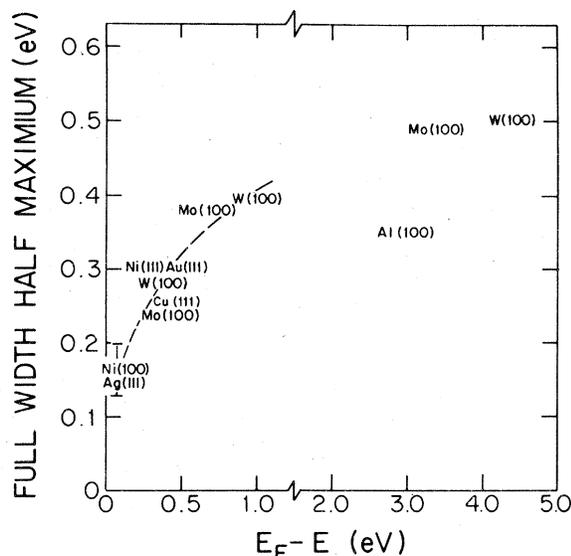
FIG. 7. Full width at half maximum (FWHM) of surface states on metals. Ag(111), Au(111), and Cu(111), Ref. 8; W(100) and Mo(100), Ref. 5; Al(100), Ref. 31; and Ni(111) Ref. 12.
