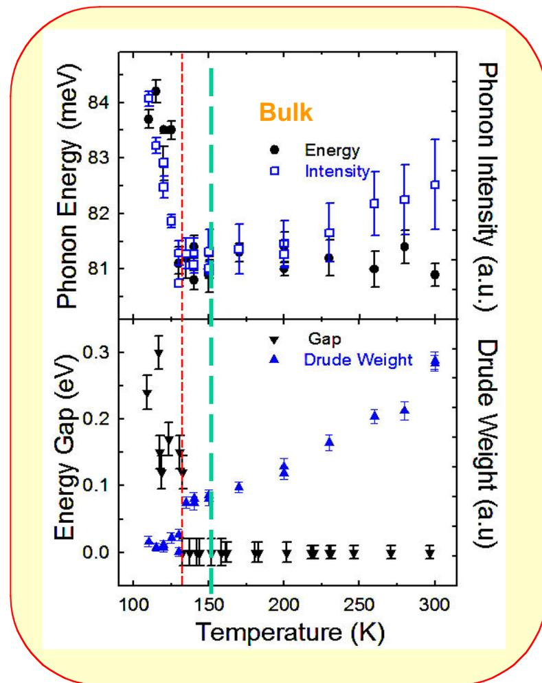
**Fig. Caption:** The top panel shows the intensity (right) and energy (left) of an optical phonon at the surface measured with Electron Loss Spectroscopy (ELS). The bottom panel displays the energy gap (left) determined with scanning tunneling spectroscopy and the Drude weight measured with ELS. The Drude weight is a measure of the conductivity of the surface. All four measurements give a transition temperature of 130K.
