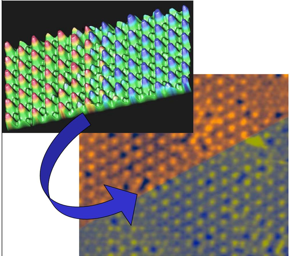
**Image above:** An artist's rendition of the STM image of a wall between two domains (red on the left and blue on the right) of the low temperature phase of Sn/Ge(111).
