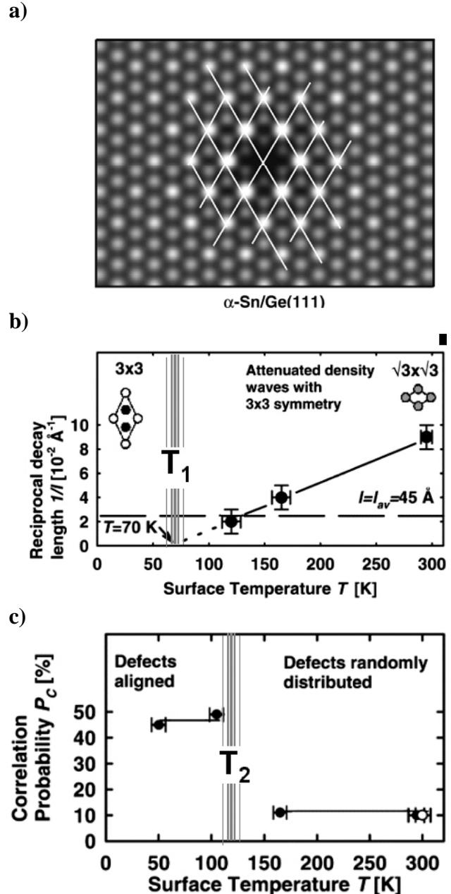
Fig. 2. (a) simulation of damped CDW from Ge defect. (b) inverse CDW decay length  $1/l(T)$ . (c) defect alignment correlation probability  $P_C$  vs. temperature.
