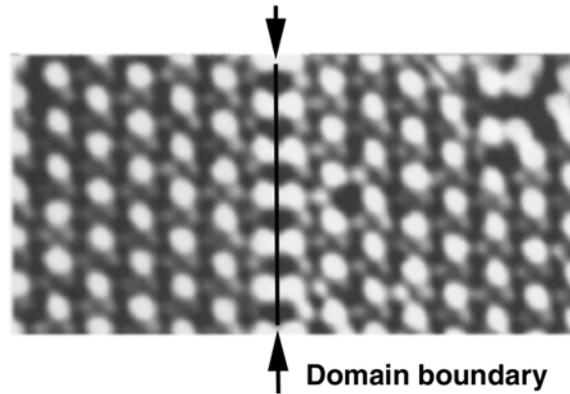
Fig. 4. STM image of sharp CDW domain wall for Sn/Ge(111) [6].
