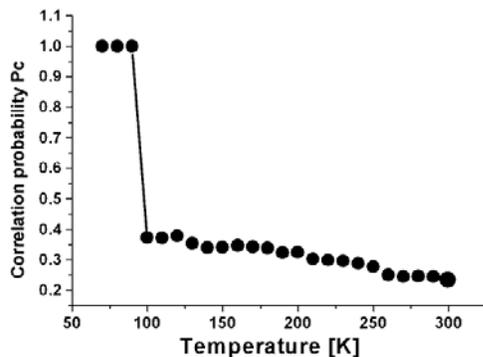
Fig. 3: Simulation of the order-disorder defect alignment phase transition
