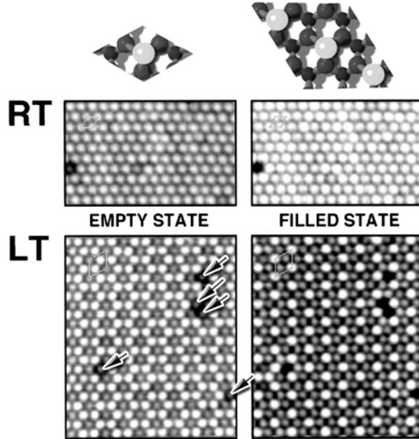
Fig. 1. Marble models (top) and STM images of the CDW transition in the  $\alpha$ -phase of the Sn/Ge(111) system (1/3 monolayer). Arrows mark Ge substitutional defects.
