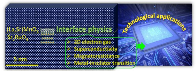
Epitaxial growth of oxide film on unconventional substrate with atomically sharp interface.
