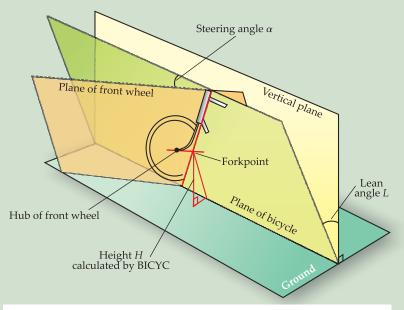
**Figure 3. A tricky trigonometrical problem.** We need to know *H*, the height of the forkpoint from the ground, for a leaning bicycle. Subroutine BICYC calculates both the vertical height and the height in the plane of the bike.
