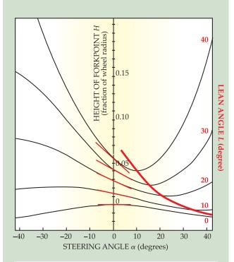
**Figure 4. Computerized bicycles.** These data, from BICYC output, show that the minimal height of the forkpoint occurs nearer to the straight-ahead position for greater angles of lean. Note also that  $dH/d\alpha$  varies linearly with lean angle *L* for small *L*. Curves, computed for typical steering geometry (20° radii front projection), are vertically staggered for clarity.
