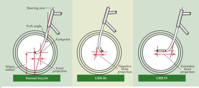
Figure 2. Front-fork geometry. On the left is a normal bicycle. The center shows URB III with reversed forks giving a negative front projection, and on the right is URB IV with extended front projection.
