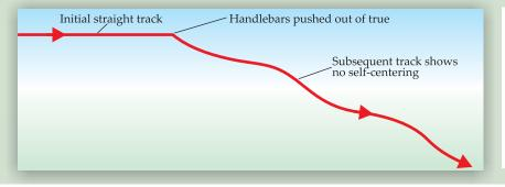
Figure 7. Self-centering? A bicycle with an "outrigger" third wheel to keep it upright was pushed and released riderless. At the point shown the handlebars were knocked out of true, resulting in a change of direction and no selfcentering. The slight wave in the track resulted from oscillations in the framework.
