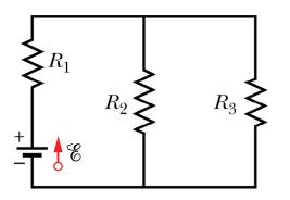
(a) (5 pts) Find the equivalent resistance for  $R_2$  and  $R_3$ .
