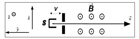
(a) (3 pts) The ions are accelerated by a potential difference of V = 10 kV. What is their final speed?
