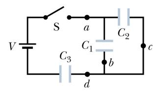
(a) (7 pts) What is the equivalent capacitance of this circuit?
