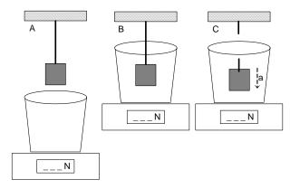
The gold is then lowered into the water until it is completely submerged, but not touching the bottom of the cup, as in Fig. B. Some water will, of course, have to spill out onto the floor (<u>not</u> onto the scale).
