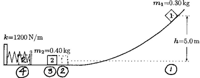
with a speed of  $v_{1,after}$ . After the collision, block 2 slides into a relaxed spring and stops momentarily after compressing it by  $x_{\text{max}}=0.40\,\text{m}$ . The spring constant (force constant) is  $k=1200\,\text{N/m}$ . Hint: It is not known if the collision is elastic!
