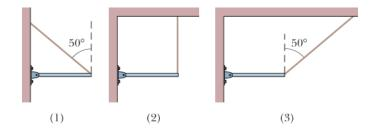
The forces on the rod are the hinge force at the left end of the rod (with horizontal and vertical components  $F_h$  and  $F_v$ ), gravity mg at the center of the rod pointing down, and tension T at the right end of the rod.
