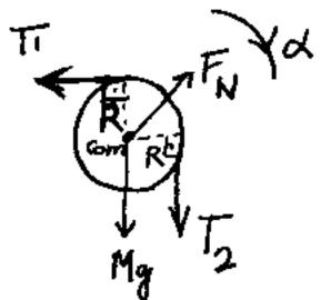
(b) (6 pts) Apply second Newton's law for  $m_1$ ,  $m_2$ , and the pulley for this situation and write the appropriate net force and net torque equations in terms of  $m_1$ ,  $m_2$ , I, R, F, g, and numerical constants, as needed.
