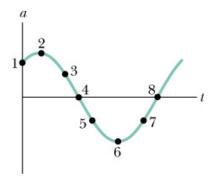
The position as a function of time x(t) for a simple harmonic oscillator is related to the acceleration as  $a(t) = -\omega^2 x(t)$ , so the plot will look opposite to the one shown above: the position will be maximum at point 2, minimum at point 6, and zero (going through equilibrium) at points 4 and 8. The velocity is maximum when the particle goes through equilibrium, it will be positive when the position is increasing (point 4) and negative when the position is decreasing (point 8).
