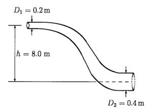
(b) (16 pts) If the pressure at the upper level is  $1.2 \times 10^5$  Pa, what is the pressure at the lower level?
