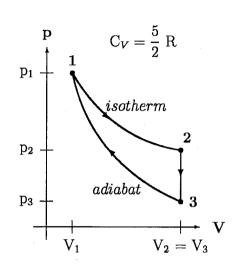
(c) (6 pts) Calculate the amount of heat absorbed  $(Q_A)$  and released  $(Q_R)$  during one cycle
