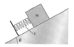
Problem 2 (20 points) A block with mass mis placed against a spring on an incline with angle  $\theta$  and an unknown coefficient of kinetic friction  $\mu_k$ ,  $\mu_k > 0$ . The block is not attached to the spring. The spring, with spring constant k, is compressed by  $\Delta x$  and then released.  $\sqrt{i} = C$ The block moves a distance  $D, D > \Delta x$ , along the incline before it momentarilly stops.
