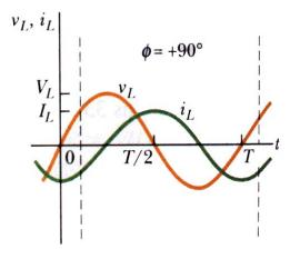
Inductors "oppose a resistance" to AC (reactance) of frequency-dependent magnitude  $\omega_d L$ (this idea is true only for maximum amplitudes, the instantaneous story is more complex).
