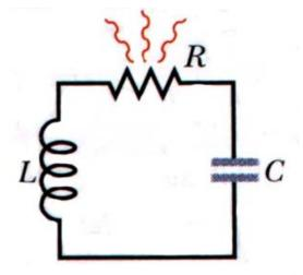
The capacitor and coil store energy, the resistor dissipates. It can be a real resistor, or just the resistance of the interconnecting wires.
