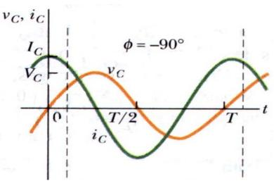
Capacitors "oppose a resistance" to AC (reactance) of frequency-dependent magnitude  $1/\omega_d$ C (this idea is true only for maximum amplitudes, the instantaneous story is more complex).
