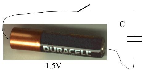
When the switch closes, electrons are moved by the battery from the top plate to the bottom one, until the potential across the capacitor equals 1.5V. Notice that in reality this is not instantaneous.
