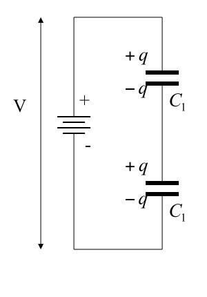
When the battery is connected, negative charges leave the top plate of C1 and move to the bottom plate of C2. The intermediate plates are disconnected from the circuit, but still get charged due to polarization.
